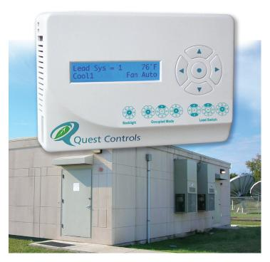
The Quest T-stat Lead/Lag Controller Model 101 is a smart control system designed to replace conventional Lead/Lag controllers that do not offer wide temperature control windows for advanced optimization of HVAC operation. The T-stat LLC controls two single stage HVAC systems to provide lead/lag operation with automatic switching based upon time. The system has a built in 2 line by 16 character display for status monitoring of the current temperature and operating mode of the HVAC equipment.
